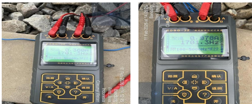
Picture 2. Track Circuit Parameter Test Results Before and After Rail Corrosion Removal
